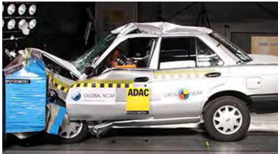
Zero-star result: passenger cell collapses and head strikes steering wheel in the Nissan Tsuru
