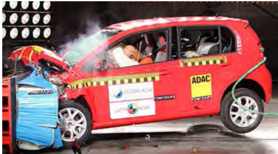
Five-star result: passenger cell stays intact and airbag protects head in the Volkswagen Up
